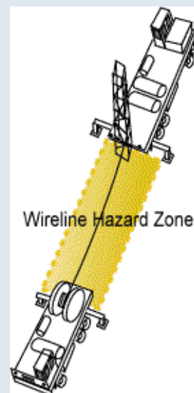
Fig. 2. Wireline hazard zone
