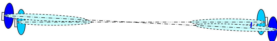
Figure 2-3: Case A—Interfering transmitter mainbeam coincident with victim receiver mainbeam
