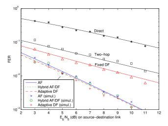
Fig. 2. FER vs. SNR, Rayleigh fading, relay at midpoint
