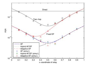
**Fig. 3**. FER vs. position, Rayleigh fading,  $E_b/N_0 = 7 \text{ dB}$
