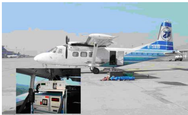
Figure 1. Y12 Chinese twin engine turboprop research aircraft used for the studies described here. Operated by the Liaoning Provincial Meteorological Agency, this aircraft carried the instrument package shown in the insert. Inlets, not shown, were mounted on an overhead aperture in the fuselage ahead of the wings.
