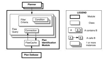
Figure 5: Class Diagram of the PlanId Framework
