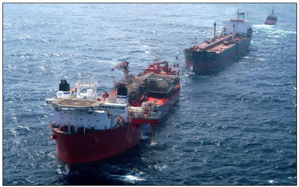
Figure 3. Actual FPSO during a Tandem Offloading Operation.
