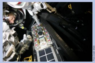
Caption: Astronaut Andrew Feustel practices installing the Fastener Capture Plate on an underwater mockup of the Advanced Camera for Surveys at the Neutral Buoyancy Laboratory in Houston, Texas.
