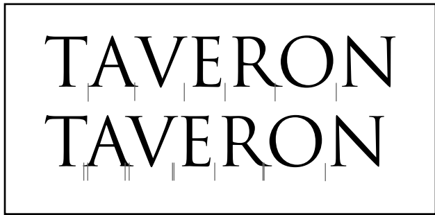
Figure 18 The top line shows Trajan™ without manual letter spacing; the marks indicate the congruent sidebearings of the letters. In the bottom line, the marks indicate the amount by which letter pairs have been manually kerned (in this case negatively kerned, or shifted so their sidebearings overlap), creating tighter, more balanced letter spacing for this title.
