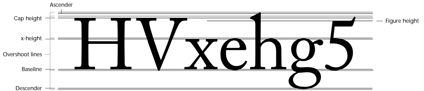
Figure A-1 Shown here are common guidelines for aligning characters of a typeface during the design process.
