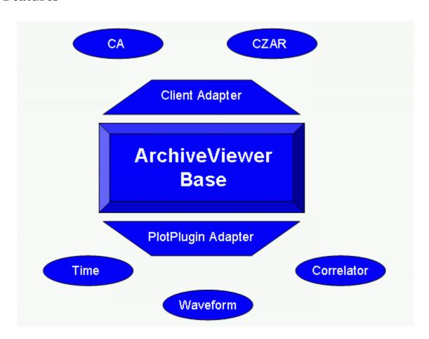
ArchiveViewer can query supported archive servers for PV data, meta information on PVs, archive settings etc. The retrieved data can take two paths: either be exported to text/binary formats, or plotted by chart widgets. Data from non-waveform, numeric PVs can also be used inside formulas, which the application eventually handles in the same way as genuine PVs.
