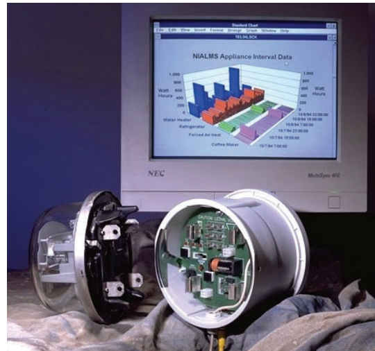
A SPEED meter ready for installation behind an electricity meter. Installation takes only about 20 minutes.
