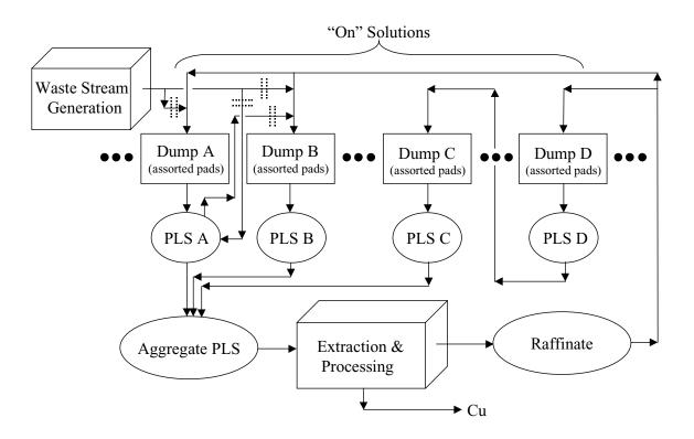
**Figure 1:** Flowchart showing the basic leaching operation and the interrelationships between the various leach solutions and ore samples. Squares represent dumps, ovals represent ponds, and cubes represent processing steps. The dashed pairs of lines near the outlet of the Waste Stream Generation indicate variable, intermittent flows.
