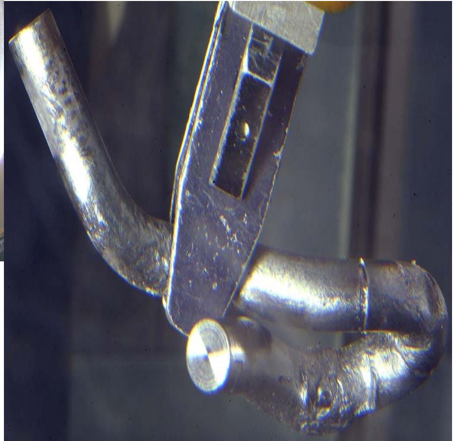
Ta-converter mounted below the UC target before irradiation
