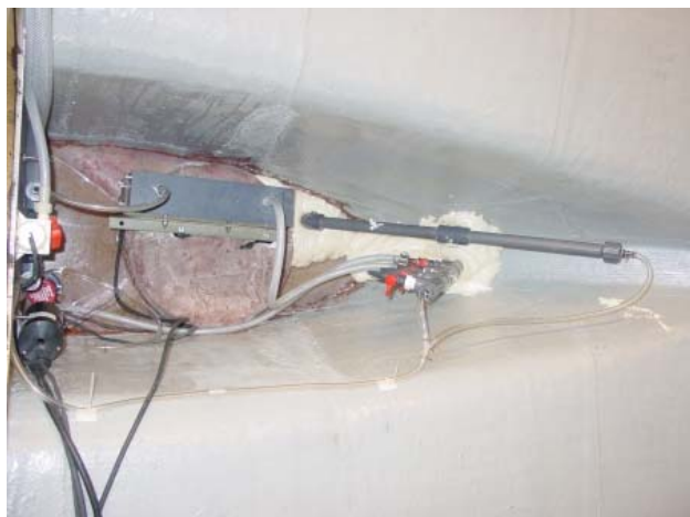
Figure 4. OASIS forward payload bay with salinity and chlorophyll sensors installed.
