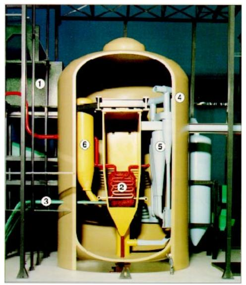
This scale model of Tidds pressure vessel shows (1) the dolomite feed system,
