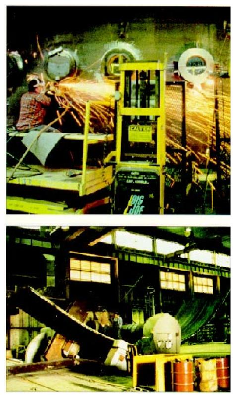
Sparks fly as a worker grinds the edges of a service opening (top). A steel plate 3 inches is bent to form a section of one of the three steel rings that were welded together to the pressure vessel shell (bottom). Prefabricated at B&Ws facility in Mt. Vernon, Indiana, the pressure vessel stands ready for removal of the top head and installation of internal components (opposite).
