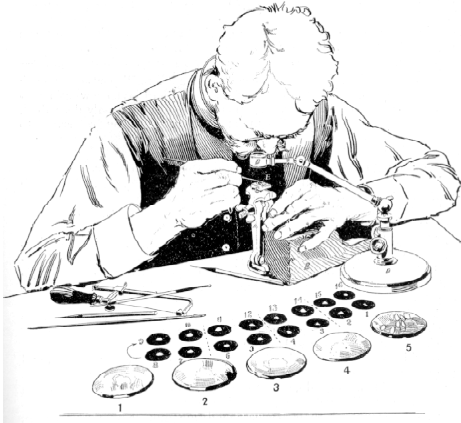
Method for removing flour from different parts of single halves of wheat grains [370]
