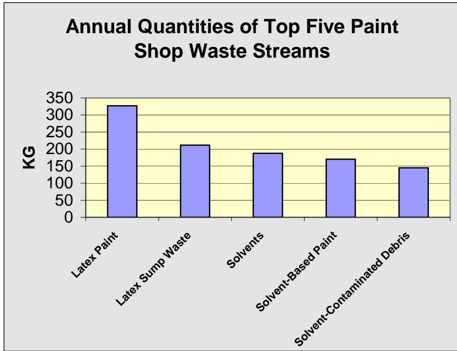
Figure 5. Quantities of Top Five Paint Shop Waste Streams.
