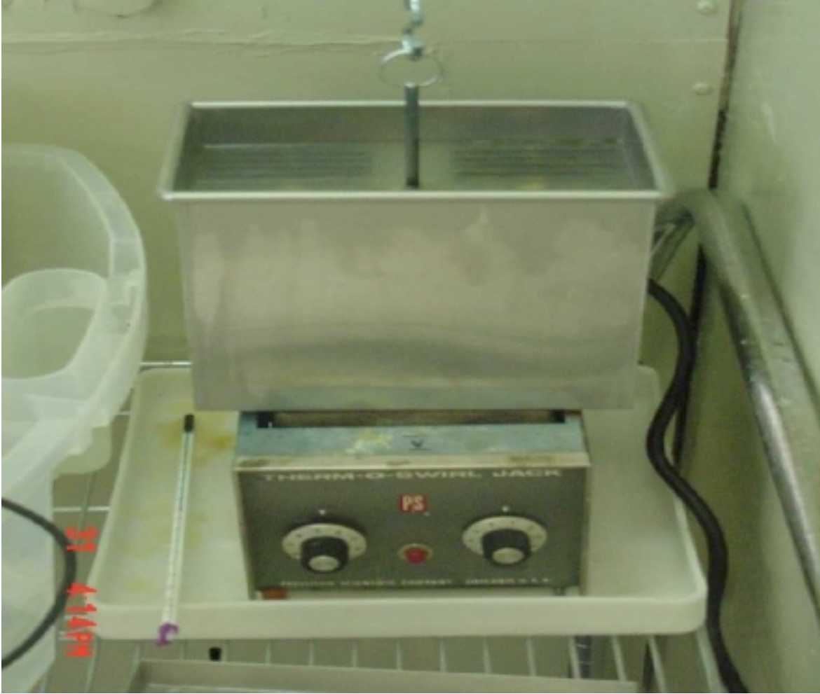
Figure 3. Cleaner Bath with Submerged Rack and Panels
