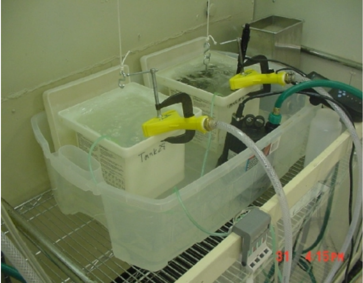
Figure 4. Rinse Tanks with Rinse Water Addition Nozzles
