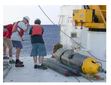
Electomagnetic streamer being deployed from the stern of the research vessel Pelican. Shown on deck are the transmitter (large body with the yellow nose cone) and two of the three receivers. The third receiver is already in the water. Pictured (left to right) are a deckhand, Rob Evans, and Alan Gardner.
