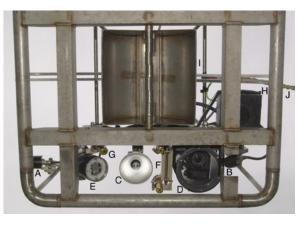
Mini SEABOSS components viewed from below: A, forward video camera; B, downward video camera; C, video light; D, digital still camera and housing; E, strobe light; F, parallel lasers for scale; G, laser for ranging; H, junction block; I, van Veen grab sampler; J, multi-conducting cable.
