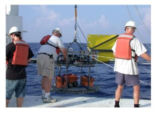
Towcam system going over the side. The frame is rigged with a camera on the bottom surrounded by orange battery packs. Electronic equipment, including a device that measures the conductivity, temperature, and depth (CTD) of seawater, sits at the top level of the frame. Strobe lights are positioned on the wings extending from the apparatus. Pictured deploying the system are (left to right) Alan Gardner, Marshal Swartz, and Rob Evans.
