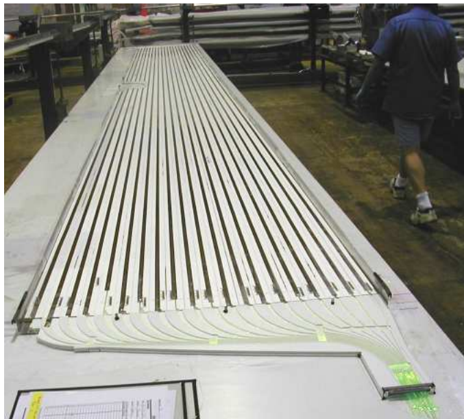
Figure 3.9: Photograph of a scintillator module before the aluminum case has been sealed. The module is 20 strips wide. In the foreground is the manifold that guides the WLS fibres to the optical connector. The extra lengths of fibre within the manifolds are often referred to as “pigtailed”. The fibres have not yet been trimmed to the connector. There is another manifold at the other end of the module to enable readout from both ends.
