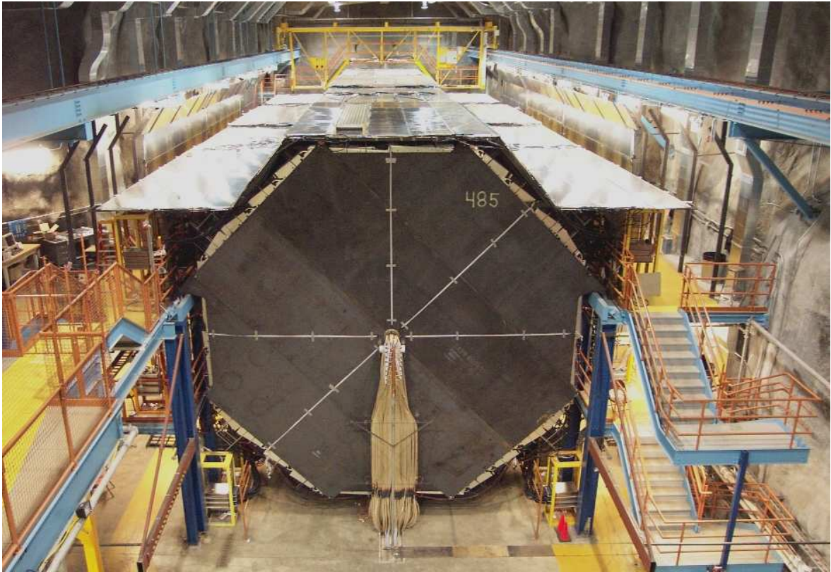
Figure 3.5: Photograph of the Far Detector. The extra planes of scintillator on top act as a veto shield for cosmic muons.
