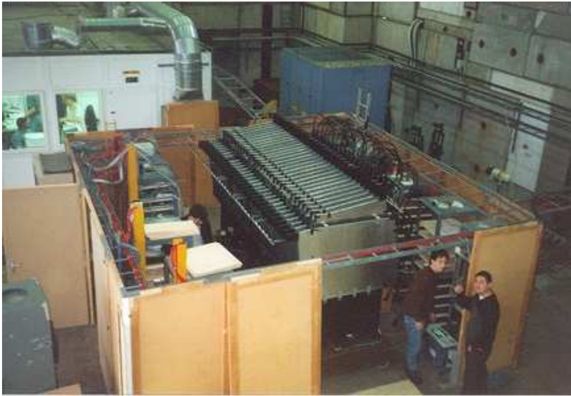
Figure 4.1: Photograph of the Calibration Detector during assembly outside the test beam area. Two humans ( \sim 6' tall) are included to give a sense of scale.
