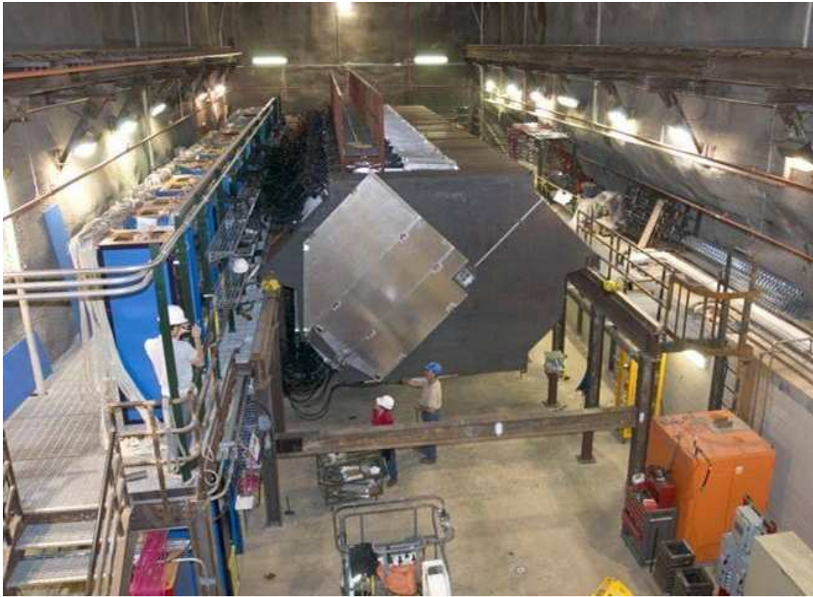
Figure 3.14: Photograph of partially constructed Near Detector. The plane at the front is partially instrumented. Photograph courtesy of K. Grzelak.
