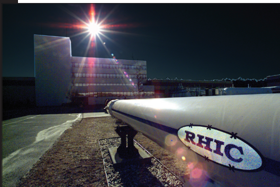
A RHIC superconducting magnet on display outside the RHIC Collider Center
