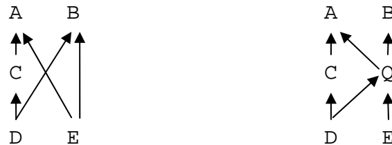
Figure 1. Subsumption hierarchies (Hasse diagrams) where arrows indicate subclass relationships ( e.g. , owl:subClassOf ). (Left) Original, manually asserted hierarchy. (Right) The Dedekind-MacNeille completion makes it clear that there exists a least common subsumer (LCS) Q that is the minimal class of all individuals with properties shared by D and E.
