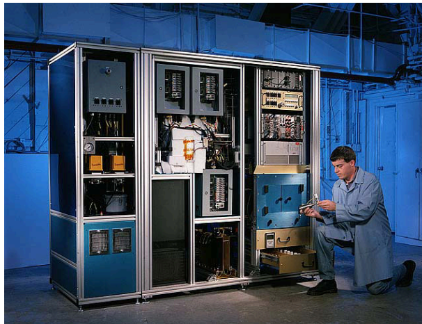
Figure 4.3. Automated Radioxenon Sampling and Analysis System
