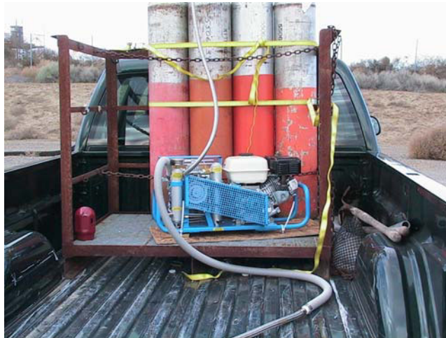
Figure 5.3. Pump and Sample Cylinders for Radon Collection
