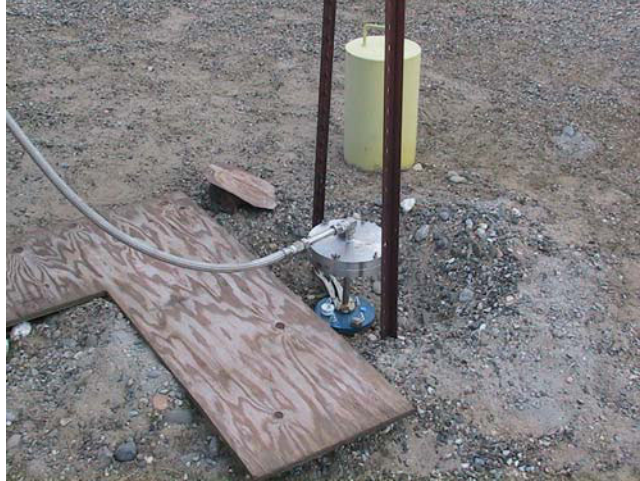
Figure 5.4. Sampling Point for Radionuclide Collection
