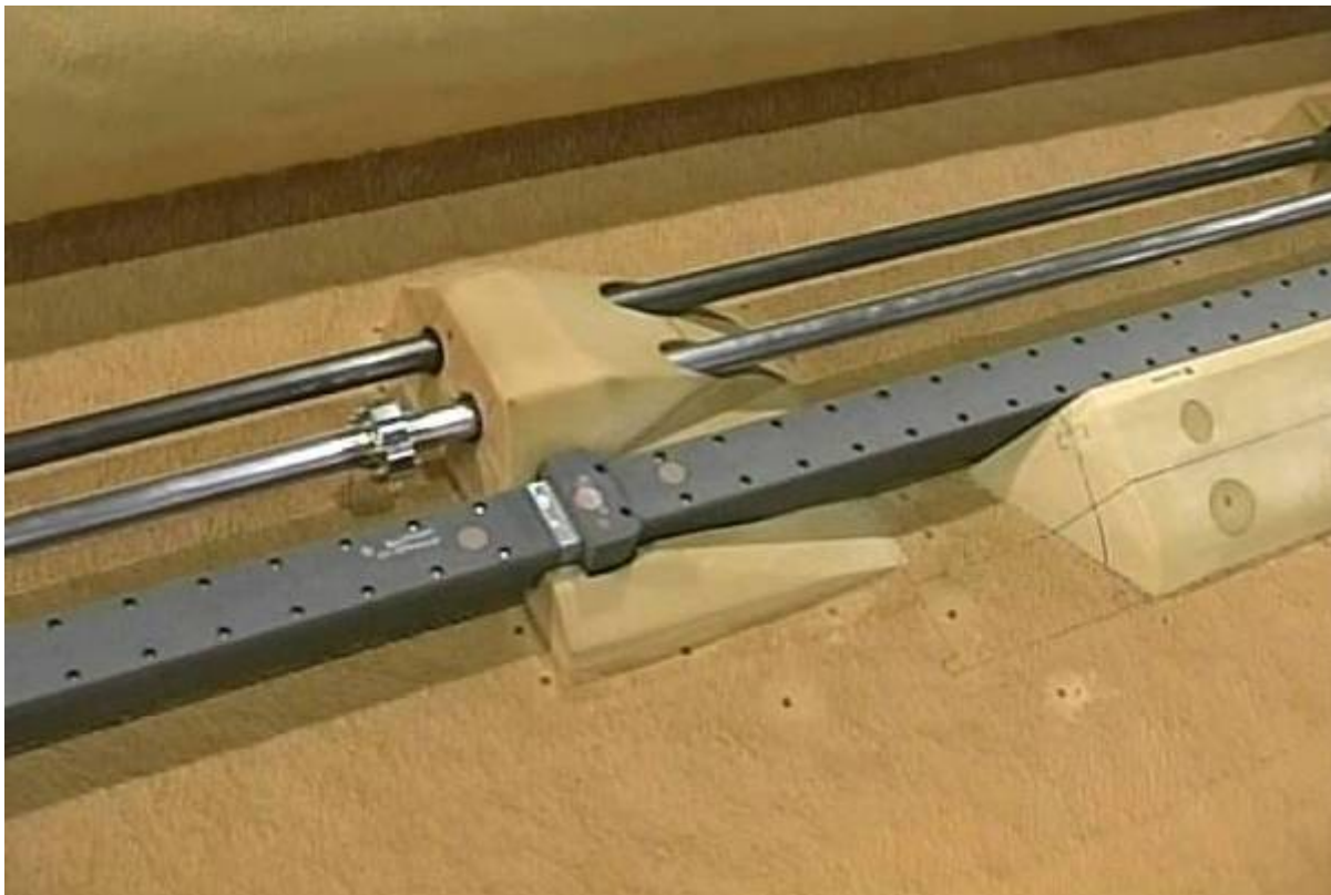
Figure 8.0-5. Repairs in the Vicinity of the ET-121 Station 1528 Ice/Frost Ramp
