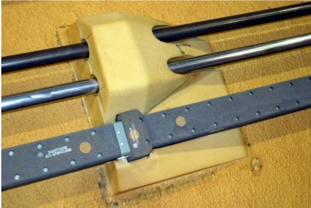
Figure 9.0-4. ET-118 Ice/Frost Ramp
