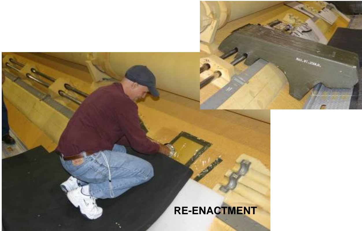
Figure 6.0-5. Re-enacted Image Demonstrating Tank Re-Work over the PAL Ramp
