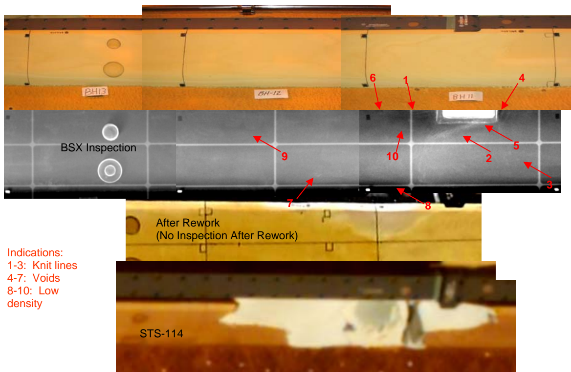
Figure 6.0-3. Backscatter Image of ET-121 PAL Ramp Foam Loss Area
