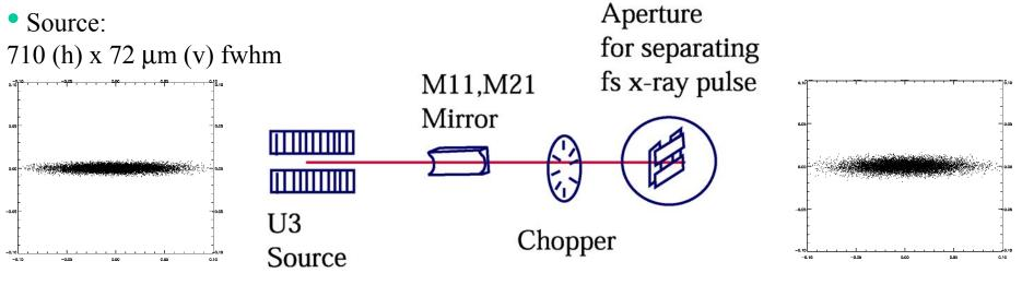
Intermediate focus: 720 (h) x 100 μm (v) fwhm 70 μm (v) for central cone
