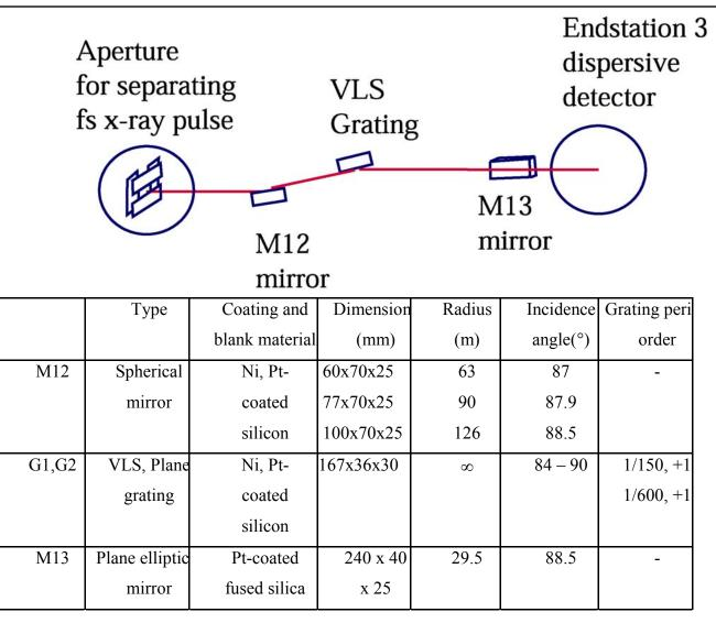
• VLS grating produces flat field spectrum at detector
