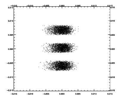
• Photon energies 849, 850, and 851 eV, 600 l/mm grating and 60 µm entrance slit.
