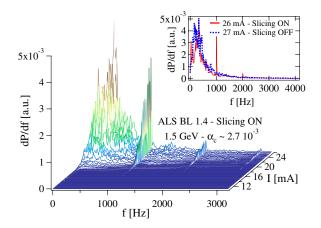
FIG. 2 (color online). Waterfall plot with the Fourier spectra of the bolometer signal for different currents per bunch. The small inset shows two spectra with slicing laser on and off.
