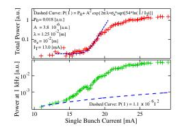
FIG. 3 (color online). Average THz CSR Power versus single bunch current. In the top panel, the measured total power is compared with theory (dashed blue line). In the bottom panel, the CSR power associated with the 1 kHz line of Fig. 2 is compared with the expected quadratic dependence (dashed blue) curve.
