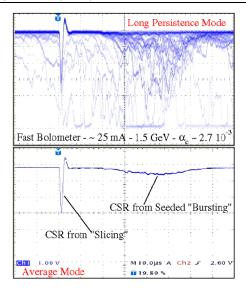
FIG. 4 (color online). The THz CSR signal as measured by a fast (800 kHz bandwidth) detector and an oscilloscope triggered with the 1 kHz slicing signal. In the top panel the oscilloscope is in long persistence mode and many individual laser slicing and burst events are observed. The lower panel shows the averaged detected THz CSR intensity.
