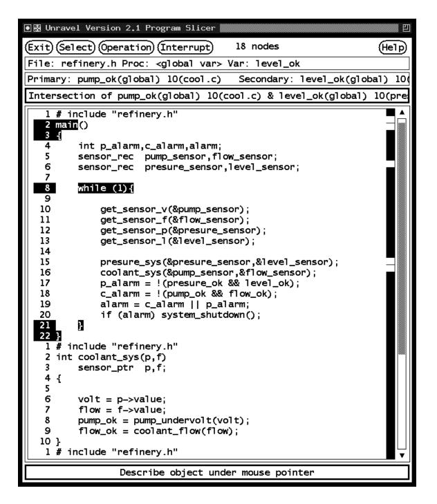
Figure 2-20: Intersection of Slices on *pump\_ok* and *level\_ok*
