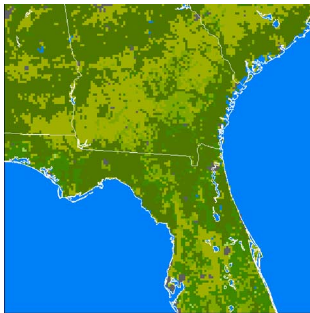
Figure 1. Horizontal model domain for the CSI JAX WRF simulations. The domain consists of 145x145 points on a 5-km non-staggered grid. Image is USGS 24-category land use class as provided via the WRF Standard Initialization package.
