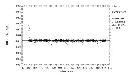
Figure 8.2.0 I3 Shipboard comparison of CTD #1 primary/secondary PRT temperatures, pressure > 1000 db.
