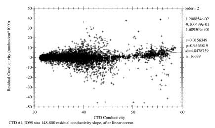
Figure 8.3.2 CTD #1 residual non-linear conductivity slope (WOCE95 stations 148 through 800).
