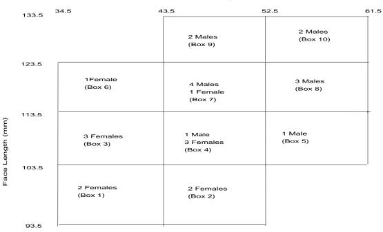
Los Alamos Scientific Laboratory Male-and-Female 25 Member Panel for Testing of Half-Masks.
