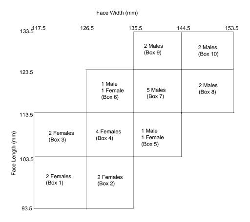
Los Alamos Scientific Laboratory Male-and-Female 25 Member Panel for Testing of Full-Face Masks
