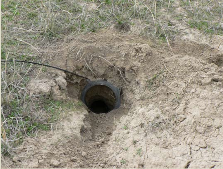
Figure 7. a) An example of the 6-inch-diameter circular antenna of a hand-held passive integrated transponder (PIT) reader over the entrance of a prairie dog burrow.
