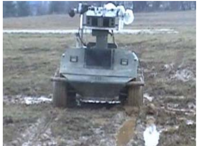
Figure 1. An experimental unmanned vehicle (XUV) navigating through a muddy grass field near General Dynamics Robotic Systems (Westminster, MD).
