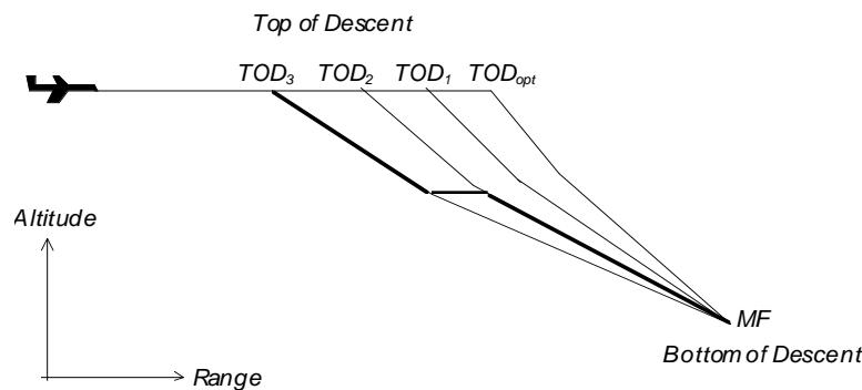
Figure 5.3 Early and Optimal (Idle) Descent TOD Locations for a Given Speed
