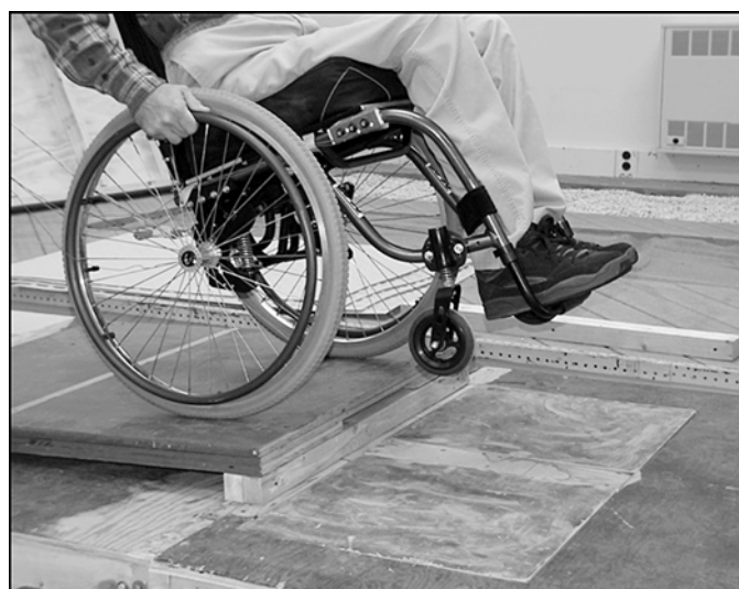
Figure 1. Example of 10 cm curb descent.
