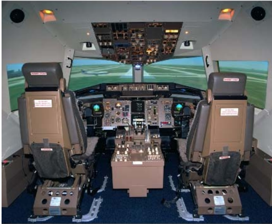
Figure 2. NASA LaRC Integration Flight Deck Simulator
