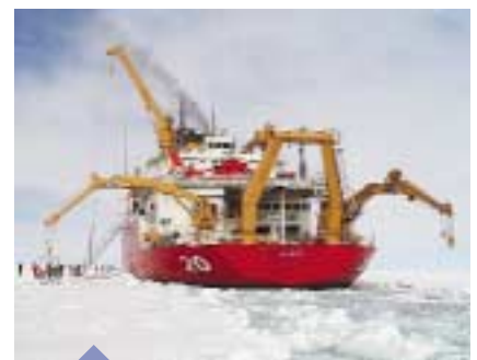
Figure 3. USCGS Healy in “spider” mode, configured for on-ice science in Baffin Bay.
