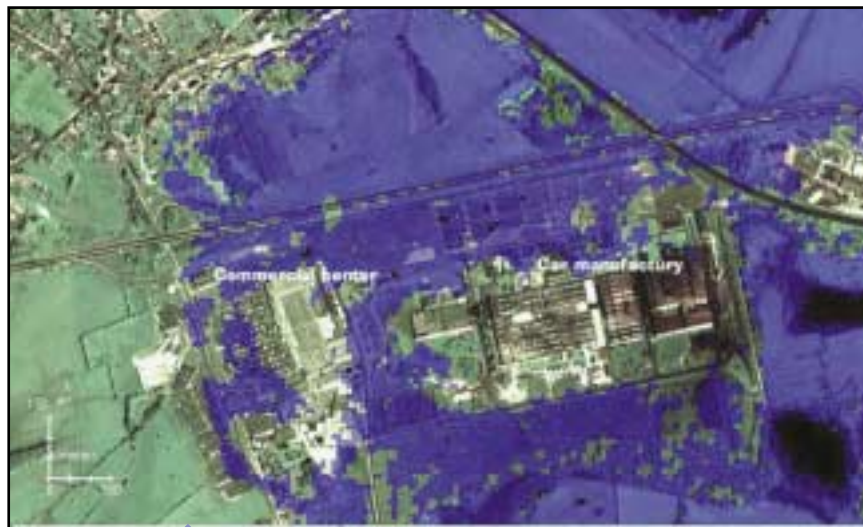
Figure 4. Damage extent and visualization based on the merging of Ikonos data and SAR derived information. Location: South Charleville, Villers-Semeuse suburb.
