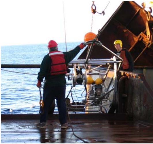
Figure 2 – Seafloor camera/sonar sled.
