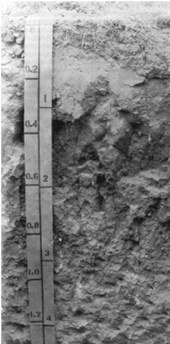
Figure 9.—Profile of Wilson silt loam. The soil is a dense silty clay which is very slowly permeable.
