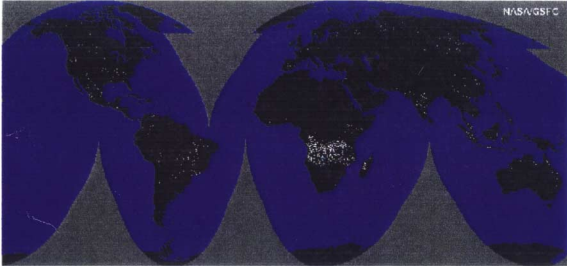
Figure 20. High temperature sources detected in 1-kilometer POES-AVHRR infrared data from June 25, 1992. Global AVHRR coverage provided by the IGBP-DIS global 1-km data set courtesy of USGS Eros Data Center.
