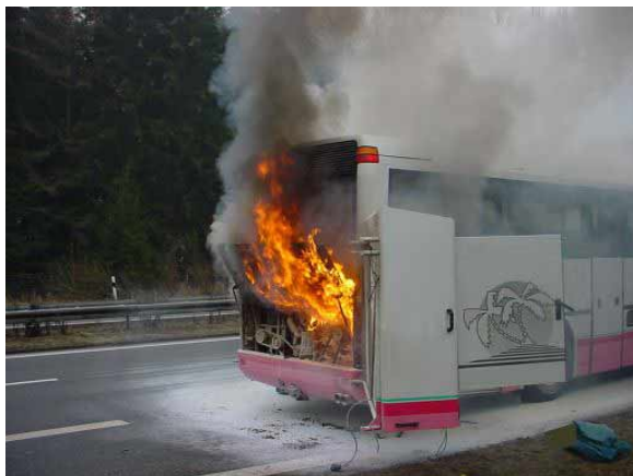
Figure 8 Engine fire after turning away the luggage box [5].
