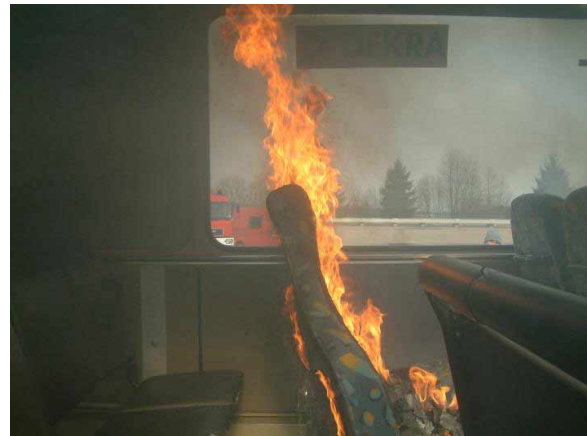
Figure 20 Seat set on fire with 0,5l of fuel (t = 10s).
