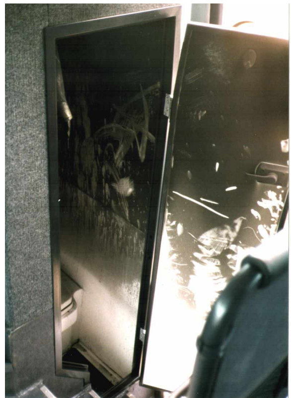
Figure 6 Toilet door with smoke-marks.
