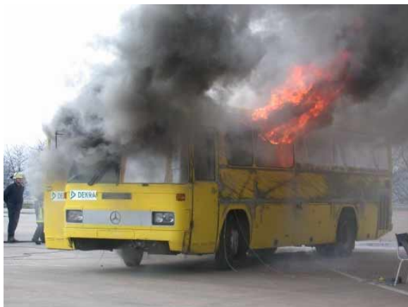
Figure 23 Breaking of the side windows during the flash-over (t = 600s).
