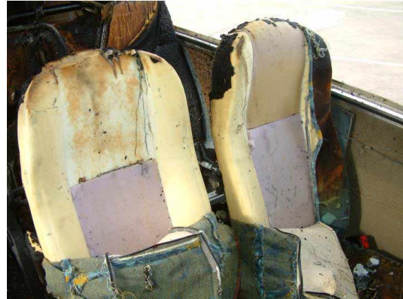
Figure 24 Seat row in front of the ignited seat. Covering removed by the fire brigade.
