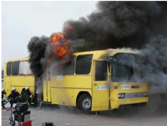
Figure 22 Flash-over and start of fire fighting (t = 600s).
