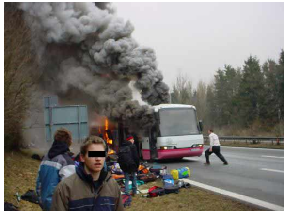
Figure 10 Fast fire spread, the complete coach is filled with thick smoke after about 10 minutes [5].
