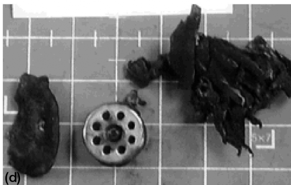
Figure 7.—Example of NASA 6001 upward flammability tests on 8 x 8 x 2.5-cm thick plastic motor and fan samples. (a) Article prior to testing. (b) Test setup, with article horizontal and igniter under case. (c) After testing at 24.6% oxygen. (d) After testing at 30.3% oxygen.
