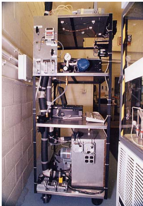
FIGURE 4. FTIR SAMPLING SYSTEM ALONGSIDE THE CONE CALORIMETER—SIDE VIEW
