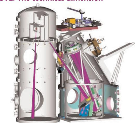
THIS COMPUTER-GENERATED illustration shows extreme ultraviolet light (EUVL) as a beam (shaded dark gray) being generated from a plasma source in the top right hand side of the apparatus, which was assembled at Sandia/California. The prototype machine was built by Sandia, Lawrence Livermore National Laboratory, and Lawrence Berkeley National Laboratory as part of a CRADA with a consortium of industry partners to support development of EUV lithography.
