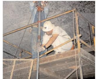
MINE CHECK — Sandian Steve Bauer (6113), on top of a scaffold in the Norton mine, runs a test to assess the mine's *in situ* permeability.
