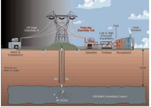
CONCEPTUAL representation of the compressed-air energy storage concept. Off-peak (low-cost) electrical power is used to compress air into an underground air-storage vessel" (the Norton mine), and later the air is used to feed a gas-fired turbine generator complex to generate electricity during on-peak (high-price) times.
