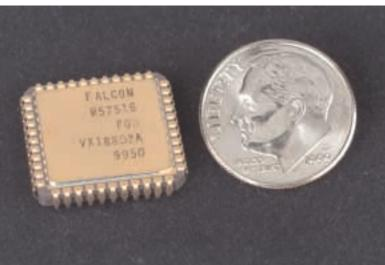
PULSE STRETCHER technique of Ken Condreva's FALCON integrated circuit, seen here larger-than-life-size next to a Roosevelt dime, makes it a high-resolution, low-cost timekeeper extraordinaire.
