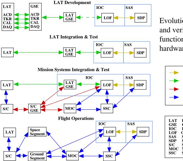
Evolutionary development and verification of IOC functions, software, and hardware
