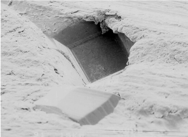
Figure 1. Diamond pull out due to weak mechanical locking inside the matrix.
