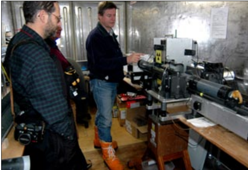
Germany's Frank Niessen, right, gives fellow ANDRILL scientists Reed Scherer and Percy Strong a tour of the multi-sensor track at the drill site. The machine can provide the researchers with details on the core's physical properties, such as density.
