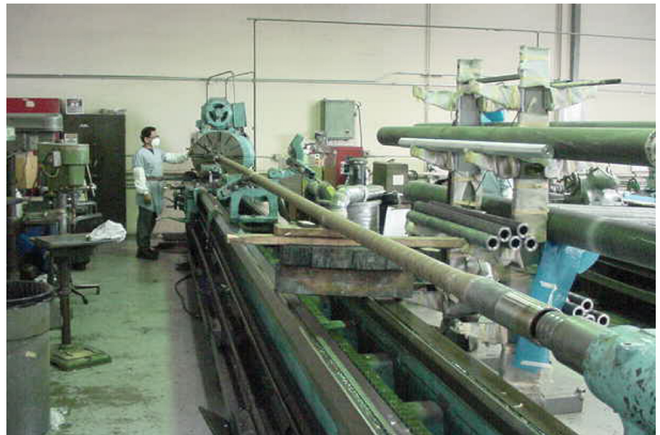
30-ft lathe for performing finish machining with SR-CDP joint in place
