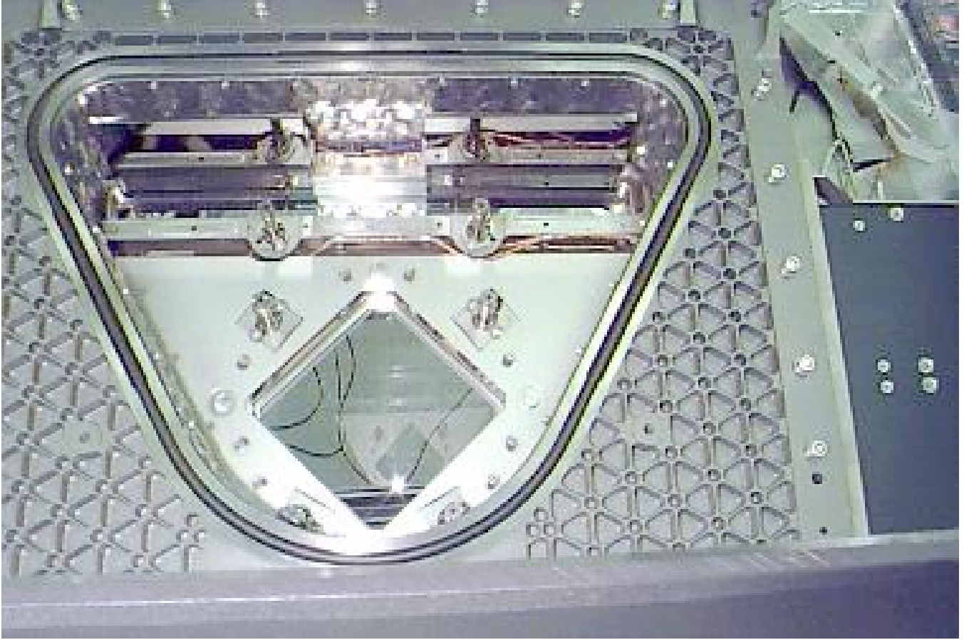
Figure 2. Picture of the High-Resolution Camera (HRC) shows the lay-out of the HRC focal-plane. The imaging detector (HRC-I) is the rotated square at the bottom; the spectroscopy detector (HRC-S), the horizontal strip at the top. An aluminized-polyimide UV/ion shield covers each detector. Just above the top edge of the HRC-S is a reflection filter for optional use to suppress higher-order contributions to LETG spectra. (Photo is from the SAO HRC team.)
