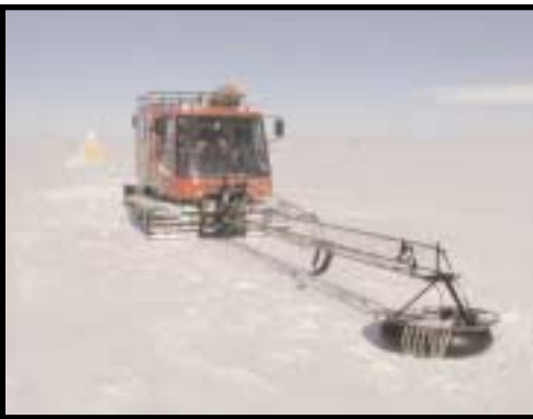
Ground-penetrating radar on 20-foot boom in front of a Pisten Bully warns of crevasses.
