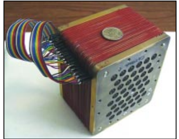
30-cell 45-cm 2 direct methanol fuel cell stack.
