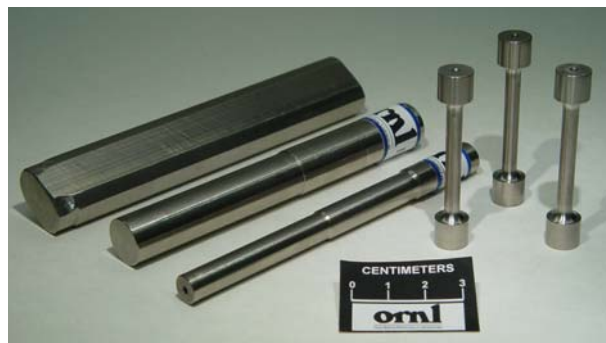
Figure 1. Extruded bars and flat stock after removing the can material and machined tensile specimens.
