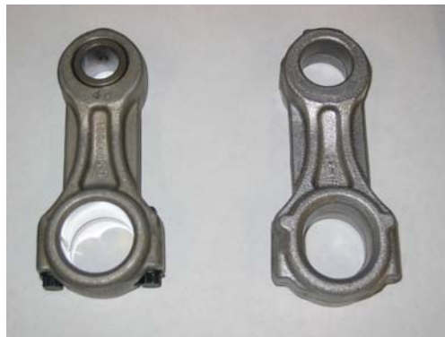
Figure 7. Machined (left) and as-cast (right) connecting rod parts.
