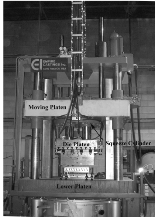
Figure 3. ASC Machine installed at Eck Industries, Manitowoc, WI
